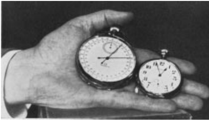
TIMING CHRONOMETER, COMPARED WITH ORDINARY WATCH
